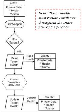
Figure 3: A view of the task flow of FireWeapon()
