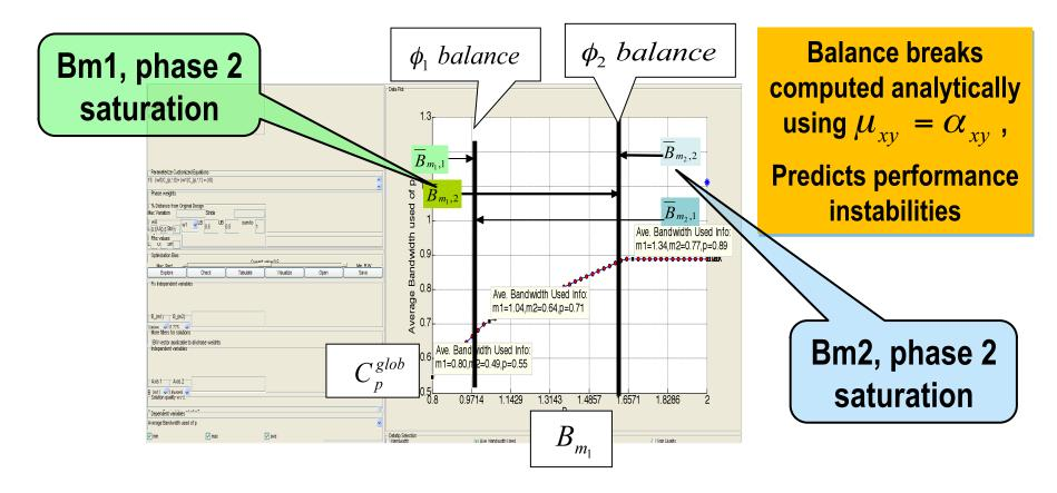
**Processor perf vs.**  $B_{m1}$ , showing 3 perf regions;  $B_{m2}$ =.775
