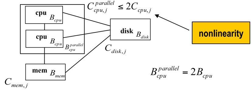
If  $C_{cpu,j}^{goal} > B_{cpu}^{max}$ , use parallel cpu model:
