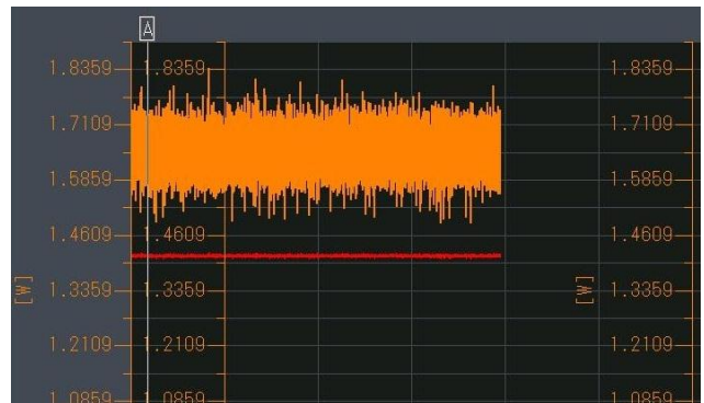
Figure8: Power consumption on RPX without power optimization
