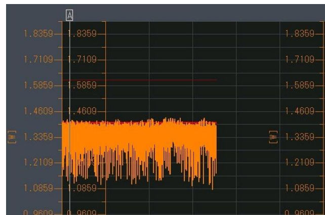
Figure9: Power consumption on RPX using power optimization
