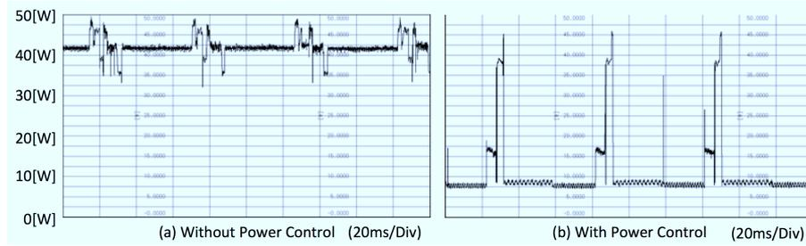
Fig. 7. Power wave of H.264 with three-cores on Intel
