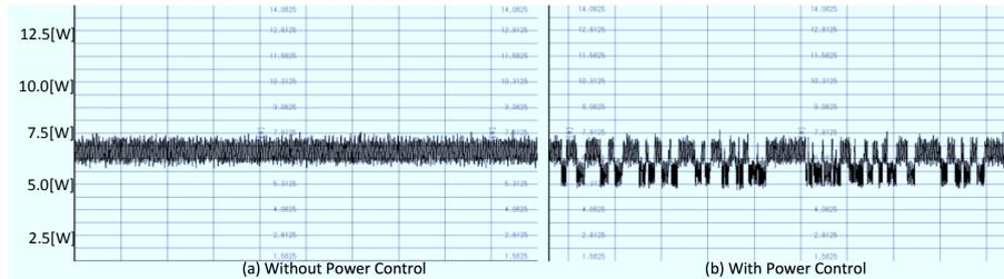
**Fig. 3.** Performance of clock gating using `MWAIT` at 800 MHz
