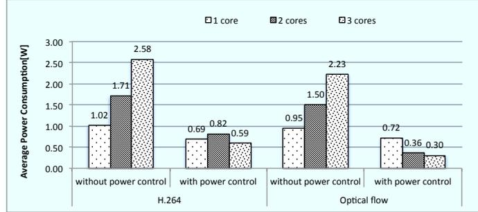
**Fig. 9.** The power consumption on the ARM CPU platform
