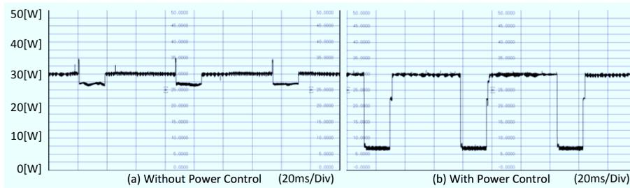
**Fig. 6.** Power wave of Optical Flow with one-core on Intel
