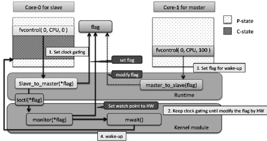
Fig. 1. Procedure for calling the MWAIT flow
