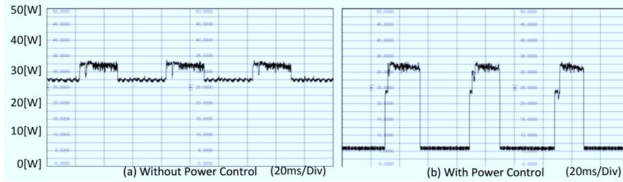
**Fig. 5.** Power wave of H.264 with one-core on Intel
