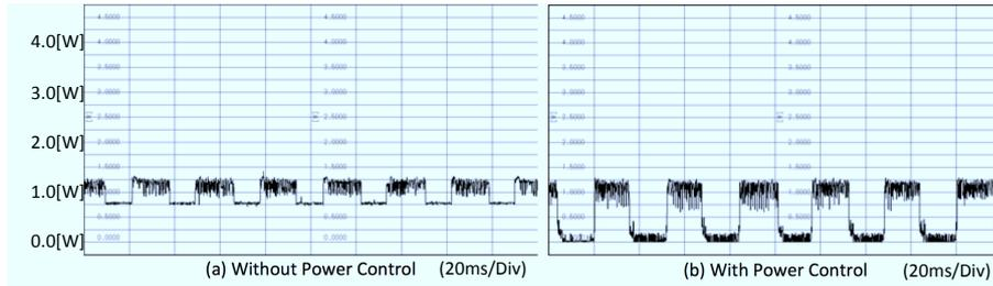
Fig. 11. Power wave of Optical Flow with one-core on ARM
