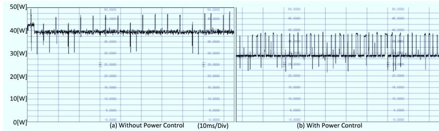
**Fig. 2.** Performance of clock gating using `MWAIT` at 3.5 GHz
