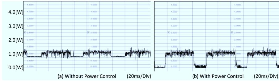
Fig. 10. Power wave of H.264 with one-core on ARM
