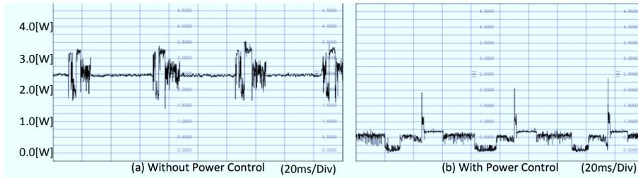
Fig. 12. Power wave of H.264 with three-cores on ARM
