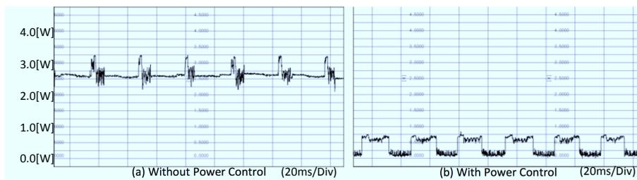
Fig. 13. Power wave of Optical Flow with three-cores on ARM
