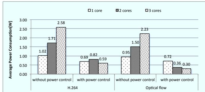
Fig. 4. The power consumption on the Intel CPU platform
