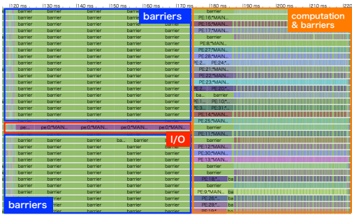
(b) The second half of the program behavior of 183.equake on 32 cores
