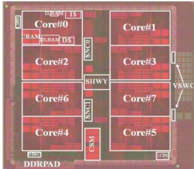
OSCAR Type Multi-core Chip by Renesas in METI/NEDO Multicore for Real-time Consumer Electronics Project (Leader: Prof.Kasahara)
