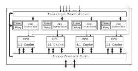
Figure 3. Block Diagram of MPCore
